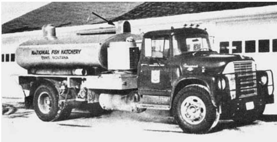
Figure 39 Aluminium elliptical tank with refrigeration unit mounted at the front. Aeration is by gas-driven pumps and pure oxygen. Note air scoops (arrow) for CO 2 removal on front and rear of tanks (Piper et al. , 1982)
