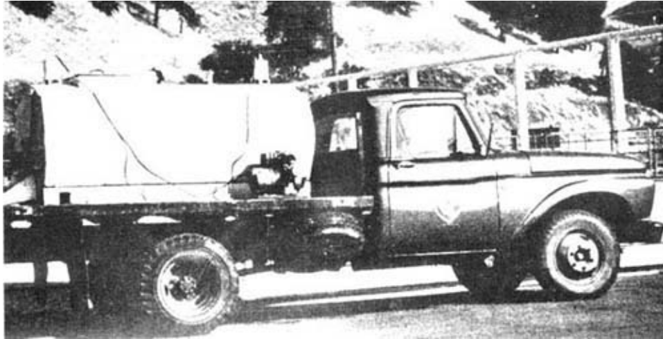
Figure 38 A 1 800-litre fish planting tank is mounted on a flat-bed pickup truck. It is equipped with a small electric pump at each end of the tank which operates from a generator or a heavy-duty truck battery, and sprays the water to the middle of the tank. It holds the temperature very constant (Leitritz and Lewis, 1976)
