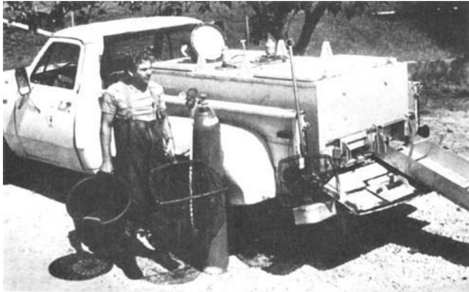
Figure 40 Small fish transport truck equipped with aerators and oxygen bottle for emergency (Dupree and Huner, 1984)
