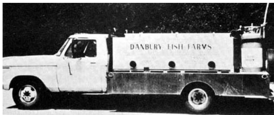
Figure 44 A fish transport vehicle equipped with liquid oxygen supply, oxygen flow valves, agitators, side ramps, and lighting for night hauling (Johnson, 1979)
